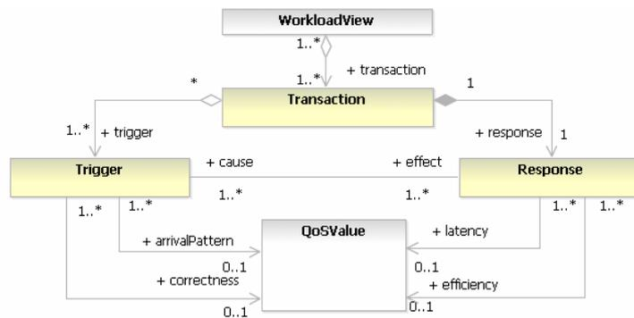
**Fig. 11.** The Workload View model of the QAM Framework
