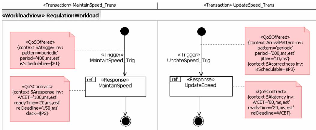
Fig. 14. A modeling example of Workload View for Schedulability Analysis
