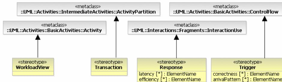
Fig. 12. The Workload Stereotypes of the QAM Framework
