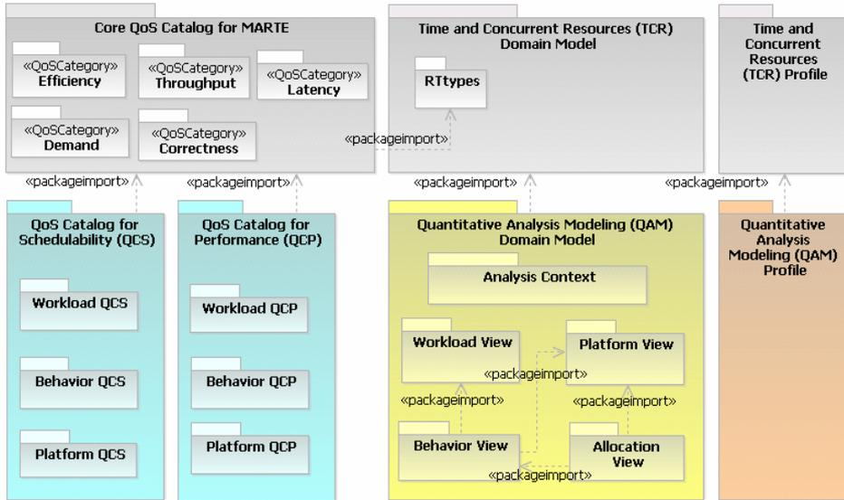
Fig. 9. Global Overview of the Analysis Framework for UML MARTE
