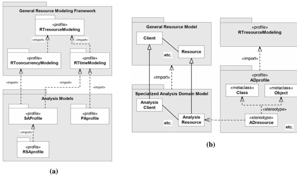
**Fig. 1.** General Structure of the SPT profile: (a) A view of the SPT packages, (b) A view of the SPT domain model and profile (Source: [11]).
