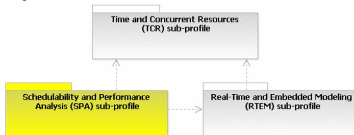
**Fig. 8.** Global Framework for the UML MARTE Profile
