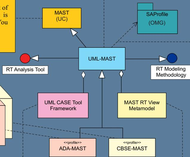
•UML-MAST models and tools can be used in combination with most of the available UML CASE tools. At present, we have a framework implemented for Rational Rose.
