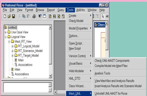
•The tools have been added to the Rose menus and are installed like if they were an Add-in. A starting Rose-framework creates a blank MAST\_RT\_View to be filled and a wizard tool helps to insert the model with a minimum of typing. The checking tool and the compiler generate a valid MAST input File.
