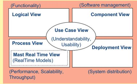
•"MAST\_RT\_View": UML view for the real-time behavior model of the system.
