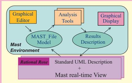
•The MAST suite is invoked directly from the UML CASE design tool. Once the RT situation has been built and compiled, it can be fed into the analysis tools and the results can be returned to the MAST\_RT\_View.
