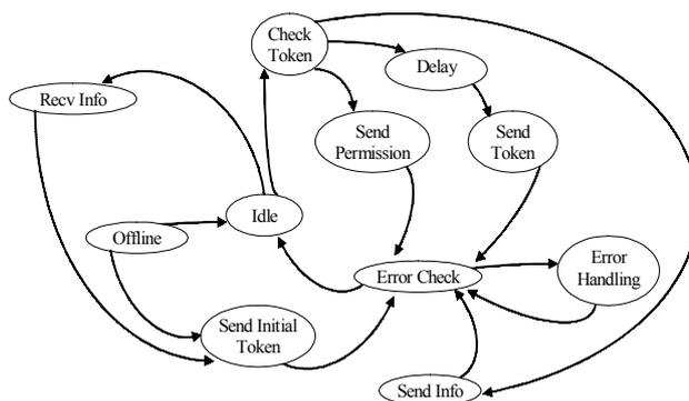
Figure 1 RT-EP state machine including faults
