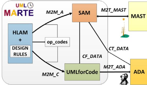
Fig. 1. Models and transformations used in our approach
